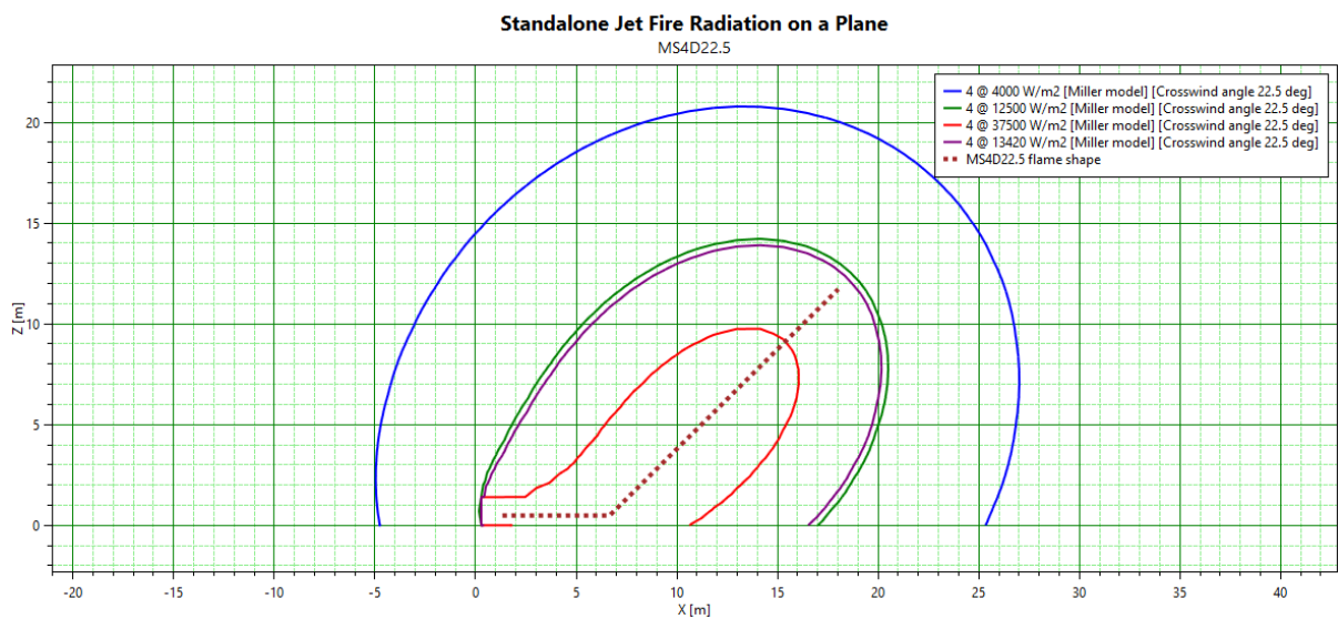
Figure 22 – Radiation contours in a vertical plane using the Miller model for Test 6
