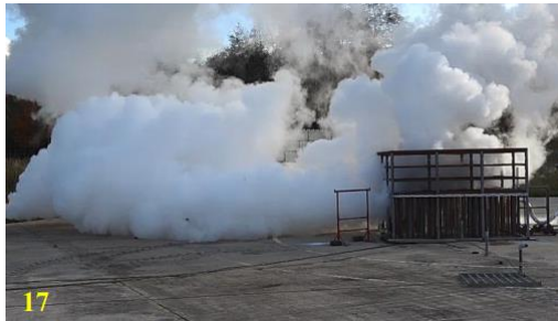
Figure 18 Flammable clouds of the test and hydrogen cloud predicted by KFX before the ignition (Test No17)
