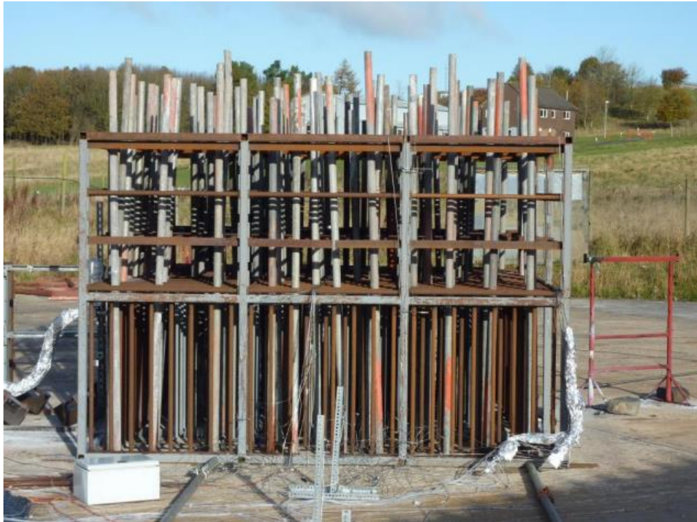
Figure 11 Photo image of the test rig with high level of congestion
