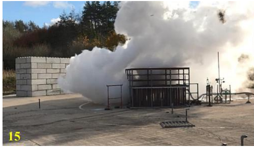
Figure 17 Flammable clouds of the test and hydrogen cloud predicted by KFX before the ignition (Test No15)
