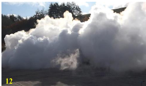
Figure 15 Flammable clouds of the test and hydrogen cloud predicted by KFX before the ignition (Test No12)
