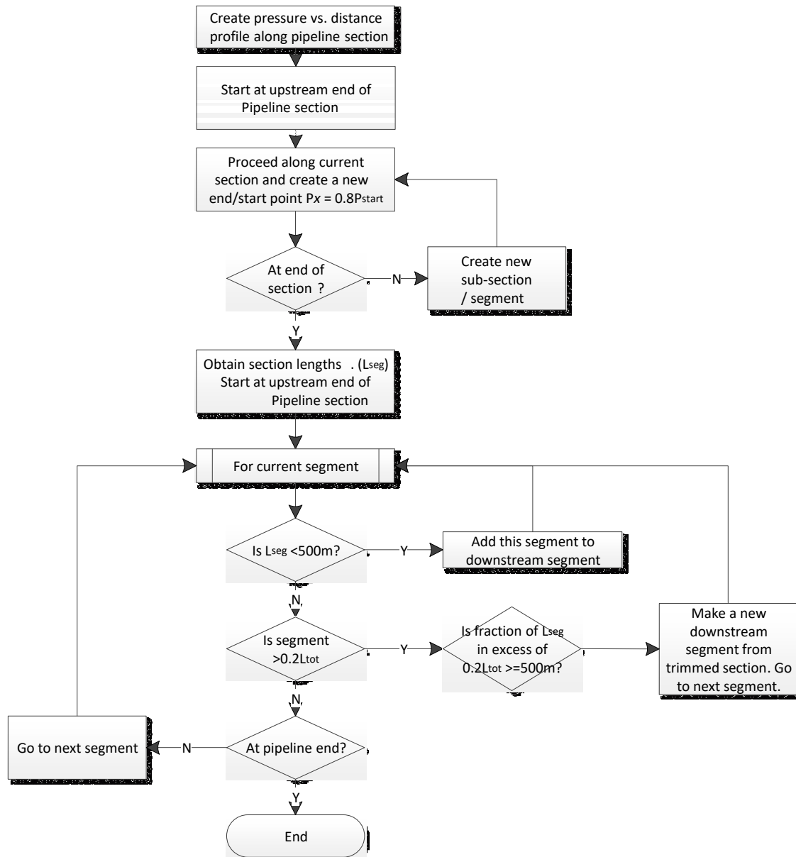
Figure 13. Automatic pipeline segmentation algorithm for a given pipeline section
