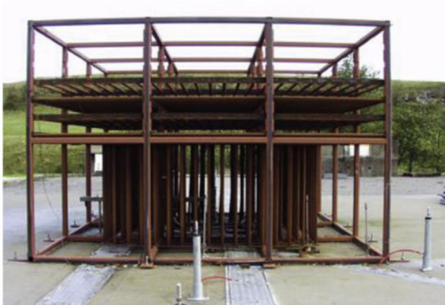
Figure 26: Shell/HSL hydrogen repeated pipe congestion test rig (4-gate configuration) [19]
