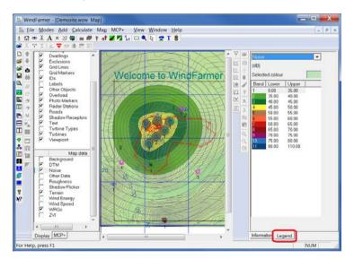
The noise is calculated from the turbine data supplied by the manufacturer, which is entered in the Turbine Studio.
