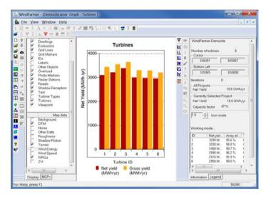
This graph shows the gross energy yield of each of the turbines plotted against the net energy yield. The Information pane to the right also indicates the overall net yield and array efficiency of each turbine.
