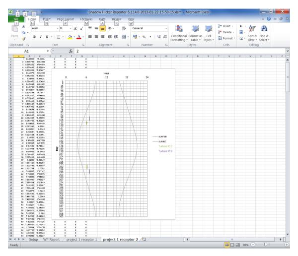
This is a plot showing when shadow flicker is possible at that receptor and from which turbine. It also indicates the sunrise and sunset times.
