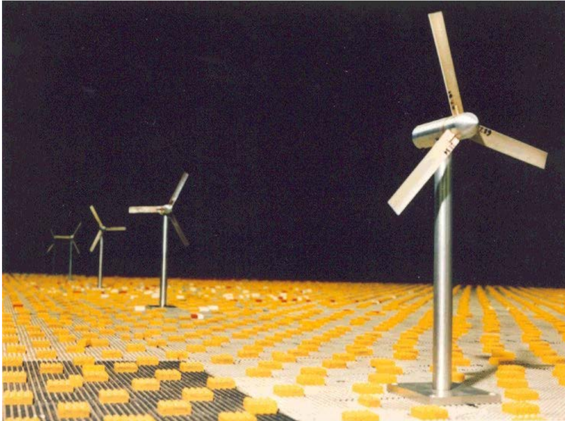
Figure 2 “Marchwood” measurements made by GL Garrad Hassan in the early 1990’s used large atmospheric boundary layer wind tunnel and fully operational wind turbines.
